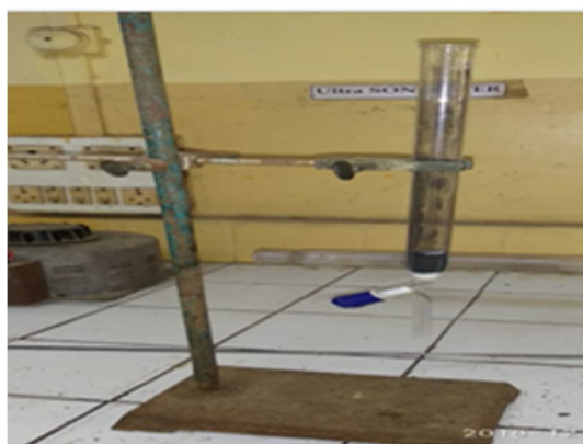
Figure 2: Set up was used to filter the polluted water.
