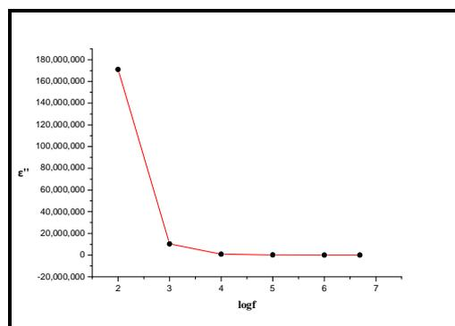
**Figure 3: Variation of dielectric loss ( $\epsilon''$ ) with log frequency of LaF<sub>3</sub>:Pr<sup>3+</sup>, Ho<sup>3+</sup>.**
