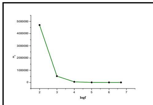
**Figure 2: Variation of dielectric constant ( $\epsilon'$ ) with log frequency of LaF<sub>3</sub>:Pr<sup>3+</sup>, Ho<sup>3+</sup>.**
