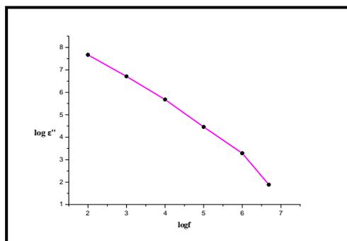
**Figure 4: Variation of log dielectric loss ( $\epsilon''$ ) with log frequency of  $\text{LaF}_3:\text{Pr}^{3+}, \text{Ho}^{3+}$ .**
