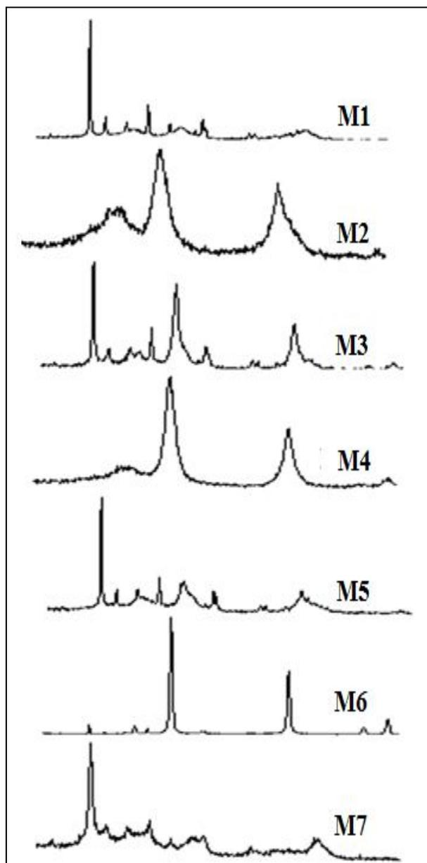
**Figure 1:** XRD patterns of calcined material (M1) MgO-Al<sub>2</sub>O<sub>3</sub> (0.2:0.8) (M2) MgO- Al<sub>2</sub>O<sub>3</sub> (0.4:0.6) (M3) MgO- Al<sub>2</sub>O<sub>3</sub> (0.6:0.4) (M4) MgO- Al<sub>2</sub>O<sub>3</sub> (0.8:0.2) (M5) MgO- Al<sub>2</sub>O<sub>3</sub> (0.5:0.5) (M6) Pure MgO (M7) Pure Al<sub>2</sub>O<sub>3</sub>.
