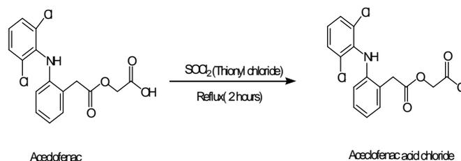
**Figure 2: Synthesis of acid chloride of Aceclofenac.**
