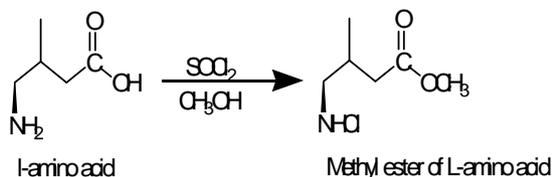
**Figure 1: Synthesis of methyl ester hydrochloride of amino acid.**
