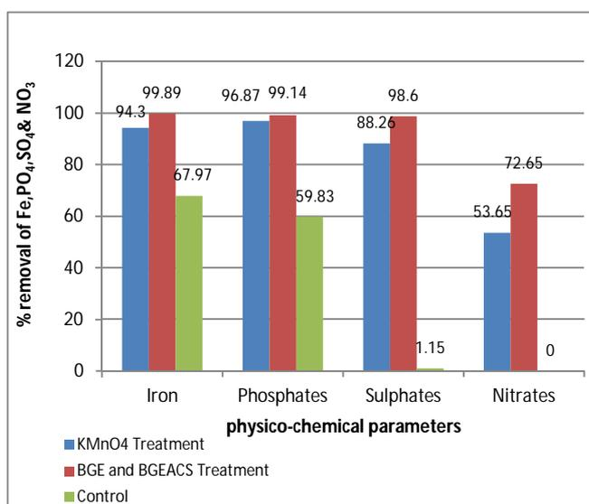
**Figure 3: Comparison of % removal of Fe<sup>2+</sup>, PO<sub>4</sub>, SO<sub>4</sub> & NO<sub>3</sub> between BGE treatment, KMnO<sub>4</sub> treatment and Control sample.**
