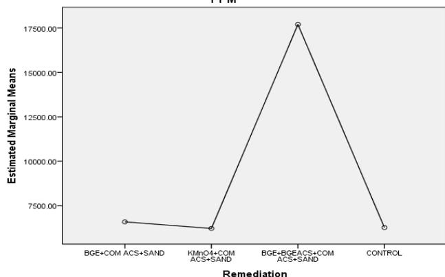
**Figure 4: Comparison of removal of Fe<sup>2+</sup>, PO<sub>4</sub>, SO<sub>4</sub> & NO<sub>3</sub> in PPM between different filtration chambers.**
