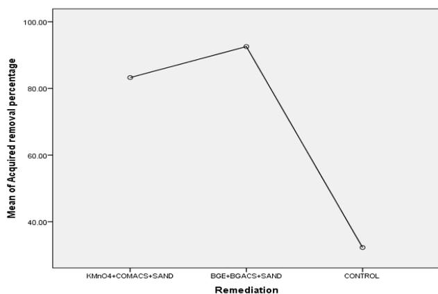
**Figure 2: Comparison of means of % removal of Fe<sup>2+</sup>, PO<sub>4</sub>, SO<sub>4</sub> & NO<sub>3</sub> between BGE treatment, KMnO<sub>4</sub> treatment and Control sample.**
